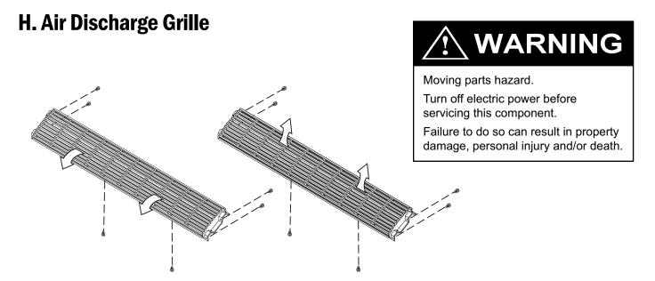
The air discharge grille can be redirected to blow air either straight up or at an angle into the room. To change the airflow direction, remove the front cover, locate and remove the six grill retaining screws. Reverse the ends of the grille and refasten the grille to the cover.
